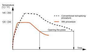
The diagram above shows the temperature curve over time when splicing an EP 400/3 conveyor belt. The short heating and cooling periods of the WK system are apparent when compared to the conventional vulcanization procedure.
