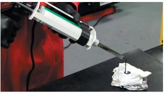
7. Assemble the mix tip onto the cartridge, depress trigger of gun to dispense a small amount of REMA GOO and then discard before using REMA GOO on belt for repairs.
