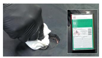
1. Clean and remove all dirt and debris from conveyor belt surface with an approved solvent and clean rag using the solvent sparingly. Do not saturate the rag or area to be cleaned.
