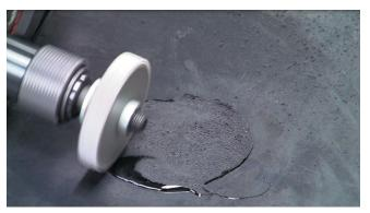
10. Let the repaired area cool to ambient temperature, if heat was used, and remove all duct tape or damming material and grind repair area smooth if needed or use a razor knife to cut the REMA GOO flush with the belting covers.
