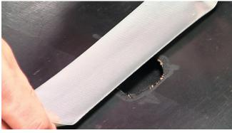
4. When REMA GOO is to be used on a hole through the conveyor belt, bevel both top and bottom covers around the hole and clean thoroughly as indicated above. Then use a polypropylene sheet or duct tape to seal bottom of hole before applying REMA GOO. You may also use Round or Diamond Shaped Repair Patches (preferred).
