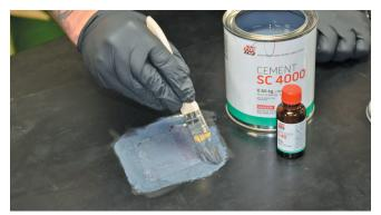
7. Apply mixture of SC 4000 Cement/ER-40 Hardener to the prepared area; rubbing it in vigorously. Let dry until the coating is slightly tacky. Test tackiness with the back of your finger (wearing gloves).
