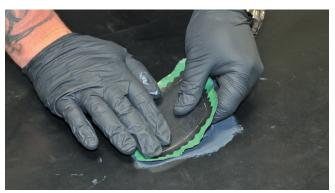
9. Apply diamond patch to prepared area; when applying the patch, both surfaces must still be slightly tacky when tested with the back of your finger (wearing gloves)
