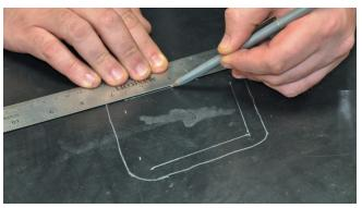
2. Trace a second marking line ½" inside the first outline, rounding off the corners.
