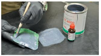
8. Apply a second coat to prepared area, as well as the back of the diamond repair patch after removal of the backing foil, with the same mixture. Allow to dry again until slightly tacky.
