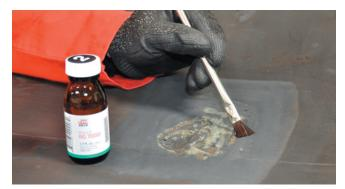
5. Apply RG 7000 Primer to prepared surface, ensure complete coverage of prepared area. Allow primer to evaporate. When RG 7000 is to be used on a hole through the conveyor belt, bevel both top and bottom covers around the hole, clean thoroughly as indicated above, and apply RG 7000 primer to prepared area. Then use duct tape to seal bottom of hole before applying RG 7000.
