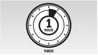
10. RG 7000 should be left completely undisturbed for the first hour after application. Equipment may be placed back in operation after 1 hour.\* Physical properties continue to develop during first 24 hours.
