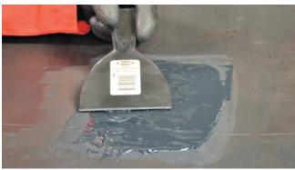
8. If belt is on an on incline, continue to work RG 7000 until thick enough that it doesn't sag, about 2-4 mins after mixing completed.
