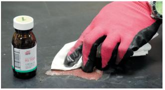
4. Use clean section of cloth to wipe buffing remnants from repair area. If area was contaminated, use solvent to clean as needed, allow to dry before proceeding.
