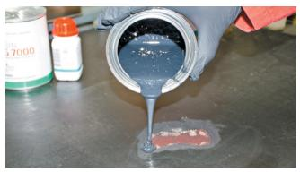
After completing the mixing, RG 7000 is pourable for 1-2 minutes.\* To ensure the best adhesions, RG 7000 should be poured onto the belt immediately after mixing.
