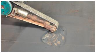
3. Prepare the surface using a buffing tool to achieve a rough profile and remove any loose material. Use the buffing tool at low speed to create a beveled edge around the damaged area.
