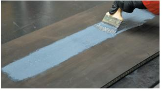
6. Apply "tack" coat to prepped surface and to the back of the repair strip.
